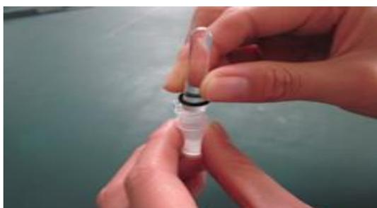
8) Remove the interface. Make sure that the reference membrane is smooth and not damaged. See the following figure:
