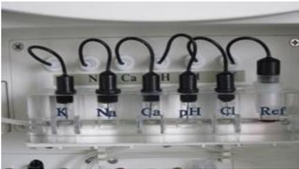
2) Loosen the fixing nuts of the electrode assembly and take out the reference electrode. See the following figure:
